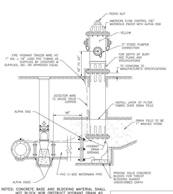
NOT BLOCK NOR OBSTRUCT HYDRANT DRAIN AS SHOWN IN AWWA MANUAL M 17
